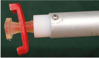
To adjust the alignment; unscrew the small screw that holds the end into the tiller cross bar and slide the white nylon spacer in or out as desired. DO NOT slide the rubber flex joint out of the nylon spacer. You will need to drill a small pilot hole into the nylon so you can re-screw the small screws back into the ends.
