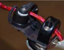
This will require some adjustment to have the keeper tight enough to hold the line in but also soft enough so that it is possible to release the cleat.
